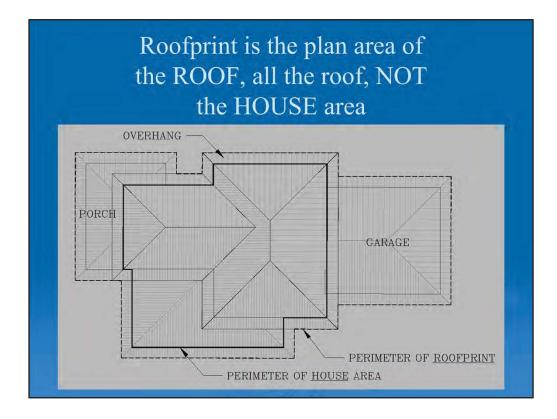
Roofprint is the area within the perimeter of a plan view of the *whole* roof.
