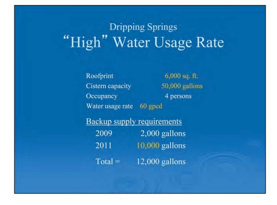
So, with water usage at this rate, to hold backup supply to a "tolerable" level, they'd have to upsize the system.
