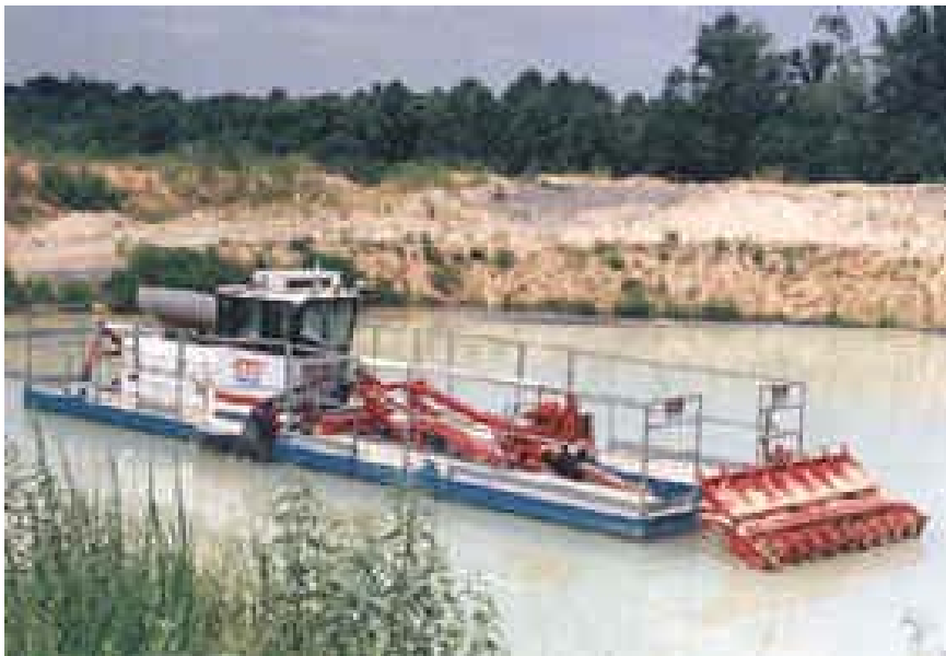
Dredging and pumping to remove sediment
