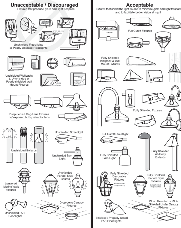
Figure D: The lights on the left are nonconforming due to inadequate shielding. Those on the right can be used in most cases; however, the mounting height and proximity to the property line may require additional shielding to prevent the luminous elements from being visible from any other property.
