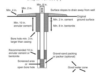
Figure 3. An example of the proper surface and annular sealing of a well.
