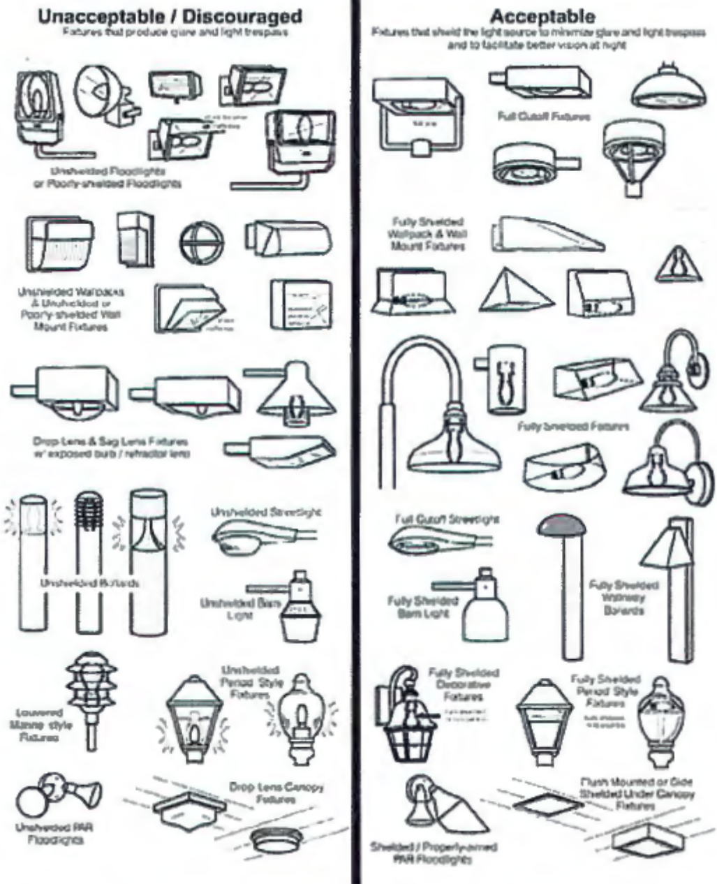
Figure D: The lights on the left are nonconforming due to inadequate shielding. Those on the right can be used in most cases. However, the mounting height and proximity to the property line may require additional shielding to prevent the lamp from being visible from other property.
