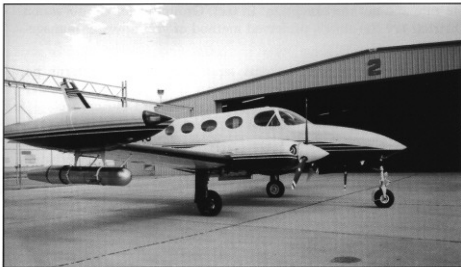
This Cessna 340 aircraft, equipped with belly racks and wingtip generators, is used for cloud seeding by three Groundwater Conservation Districts in the Texas High Plains.
